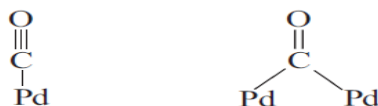
Figure 3: Different ways of molecular CO binding to the surface of the metal catalyst
